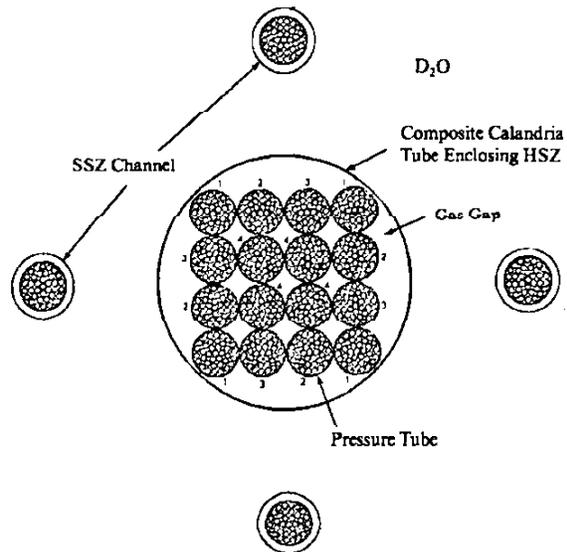
FIGURE 2 Supercell Showing Hard and Soft Spectrum Zones
