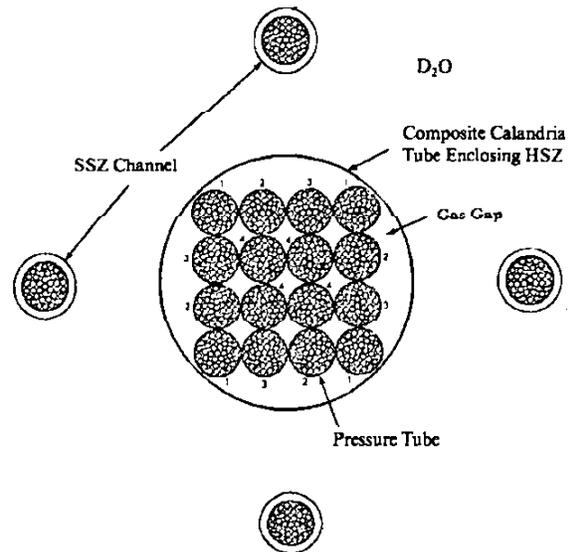
FIGURE 2 Supercell Showing Hard and Soft Spectrum
